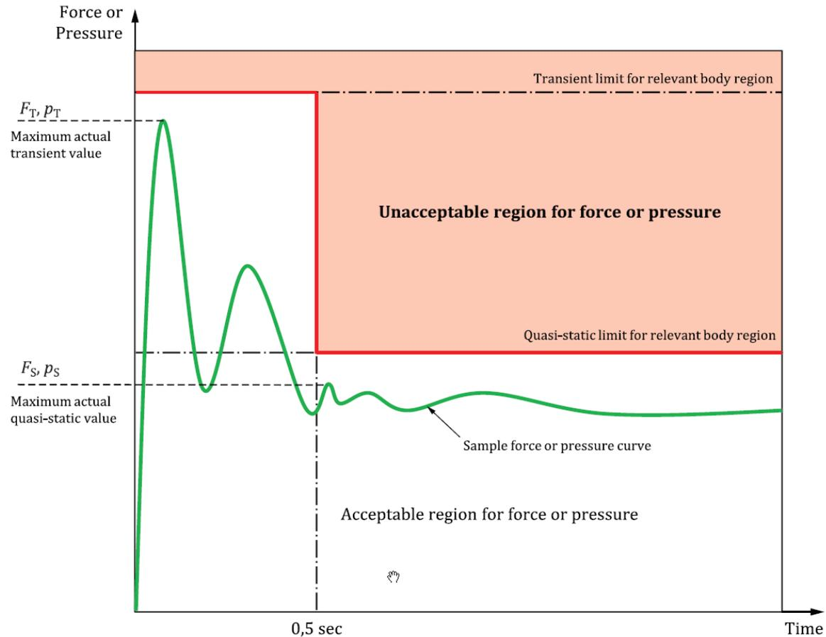
Transient contact event recording here showing both initial transient contact and continued clamping forces
