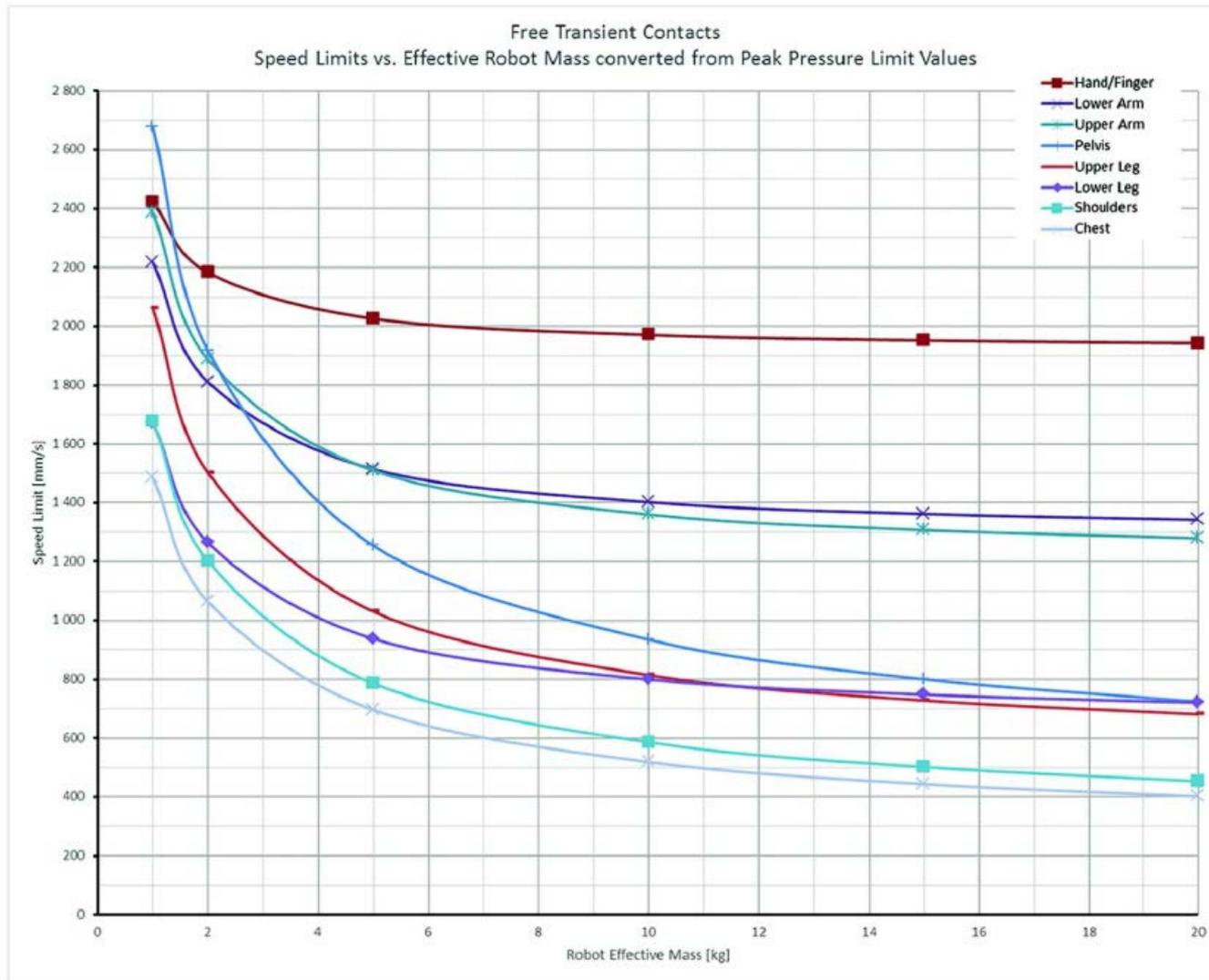
ANSI/RIA TR R15.606 Figure A.4 Graphical representation of calculated speed limit based on the body model
