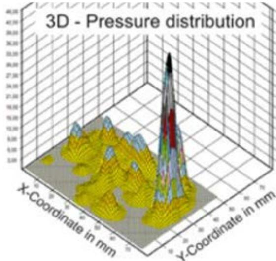
Pressure map for quasi-static test using body specific shore value pad and pressure mapping film
