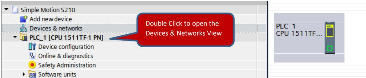
In the Devices and Networks Window, Drag and Drop in your S210 Drive model from the hardware catalog.
